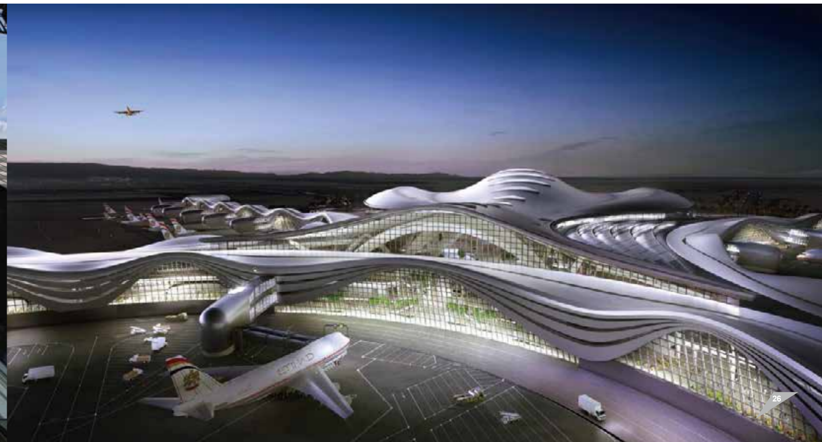
▼ Abu Dhabi Airport, UAE Glass makeup: 6mm glazed glass HS+1.52 PVB+6mm Low-E coated glass HS+12A+6mm glass HS1.52 PVB+6mm glass HS Furnace used: AG12S9042
